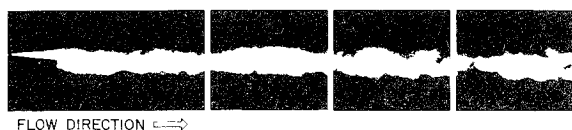
Fig. 4 Sting wake laser planograms. M_x = 2.5 , Re_{x,s} = 5.4 \times 10^7 , 0 < X/D < 26 .
